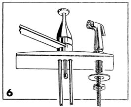
Deck mounted spray attachment model, for 3-hole kitchen sinks. Remove nut and washer from spray mount support located on bottom side of faucet.
