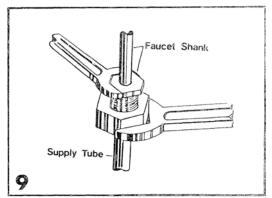
Connect both hot and cold tubes to the supply lines from the wall or floor. Left-hot, right-cold. Using care, take one wrench and hold hex of faucet adapter on supply tube and another to tighten nut on water supply line from floor or wall. DO NOT OVER-TIGHTEN!
