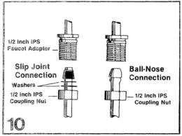
Make connection to your supply line using either a slip joint or ball-nose type supply tube. The flexible type supply tubes are available which makes for a quick, easy installation. The shank adaptor on the faucet supply is 1/2 inch IPS.
