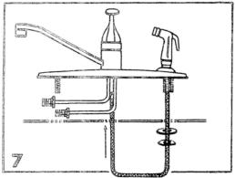
Push hose down through right-hand hole of sink. Slide washer and nut on spray hose underneath sink. (Do not fasten until Step 8.) Bring hose up through middle hole of sink deck and attach to spray hose nipple.
