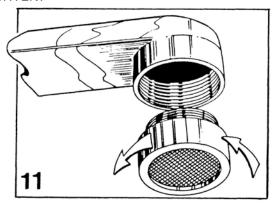
After installation remove aerator and turn faucet to a full water mix position. Turn water supply on and flush both hot and cold lines. On spray models, check spray operation for leaks.
