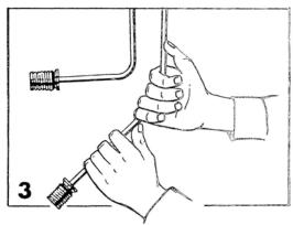
Carefully straighten copper supply tubes on faucet. This can be done by placing thumbs in back of bend and carefully straighten tubing, taking care not to crimp copper supply tubes.
