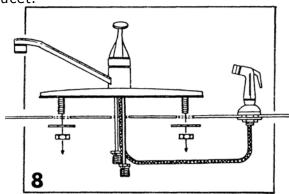
Feed straightened copper tubes and entire faucet unit down through the kitchen sink deck holes. Fasten in place with mounting washers and nuts provided. Trim off excess plumber's putty, if used, from around faucet.
