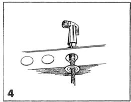
For models with spray attachments only: Attach spray mount support unit in far right hole of kitchen sink.
