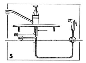
Push hose down through support unit and up through second hole from left. Attach hose to spray hose nipple on underside of faucet.
