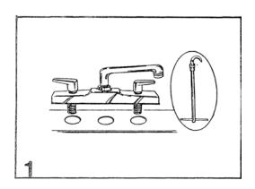
Shut off water supply. Disconnect and remove old faucet. Long handle basin wrenches are available to help simplify removal of old faucet nuts under sink.
