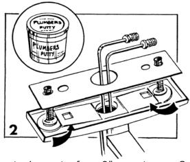
Faucet is set for 8" centers. Some models can also be set for 6" centers by moving two stud bolts on the inside of the undercover plate. Be sure base gasket is attached on bottom or discard gasket and pack bottom of faucet with plumber's putty until slightly rounded.
