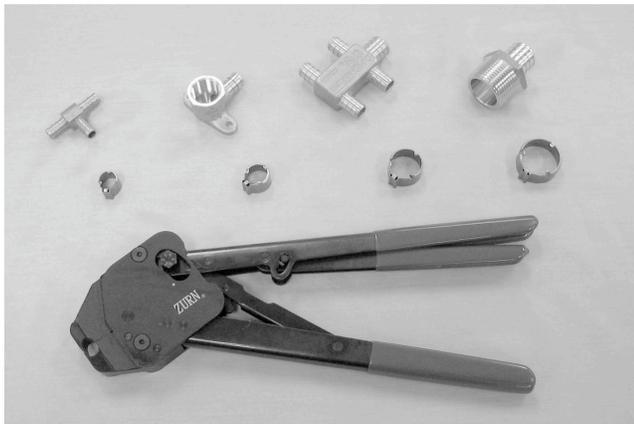
Another type of PEX connection system uses a stainless steel crimp ring to secure the fitting to the pipe. The big advantage to using this method is that one tool works with  $3/8''$ ,  $1/2''$ ,  $3/4''$  and  $1''$  pipe. Shown is the *Quick-clamp* tool, rings and a few of the many fittings available for use with PEX piping
