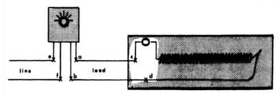
splices (C) and (B) in the single pole thermostat diagram at (E) or (F) if the double pole diagram is being followed.
